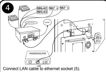
Connect LAN cable to ethernet socket (5). If RS485 hardwares will be used together with your system, connect RS485 HW cable (RJ11) to data socket (6).
