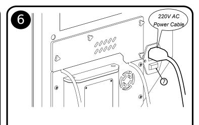
Connect 220V AC power cable to power socket then press power switch (7) to operate system.
