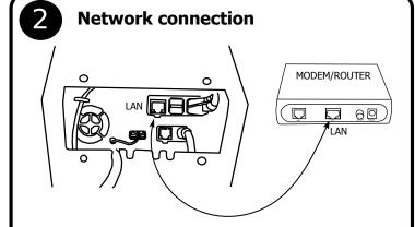
Connect ethernet cable between device's ethernet socket and your modem. You can find IP address of ticket dispenser from the LCD screen later.
