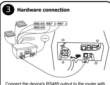
Connect the device's RS485 output to the router with Q-smart hardware cable.
