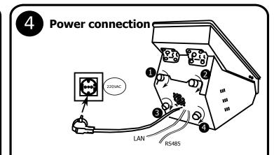
After making all connections, the cables are passed through the gaps from plastic cover as in figure when cover is closed. Reinstall 4 plastic head screws and connect device to 220 VAC.
