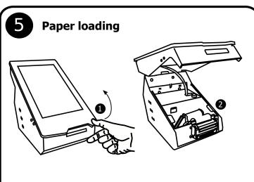
Open the cover by lifting it up from the location shown in section #1. Load the thermal paper roll in section #2 which is shown in figure.
