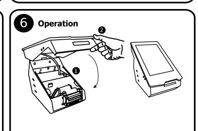
Press the On/Off button as shown by #1 for 1 second and close the cover as shown by #2 in figure.
