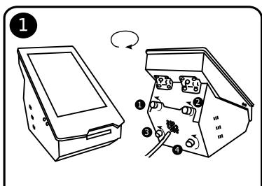
Turn back of device then remove 4 plastic head screws and remove plastic cover.
