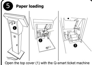
key. Unscrew the screw in section (2) and pull the rail
