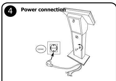
After making all connections, close the cover on the back of the device. Connect the device to 220V AC.
