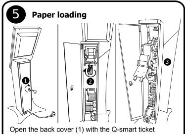
machine key. Unscrew the screw in section (2) and pull the rail towards you. Load paper in section (3).
