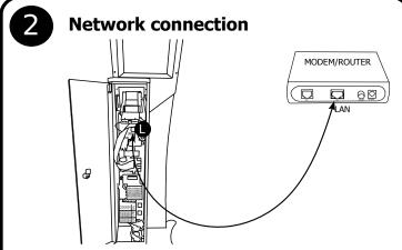
Connect the Ethernet output of the ticket machine to your modem, shown as (L) in the picture. You can find the IP address of the device on the screen when the application starting.
