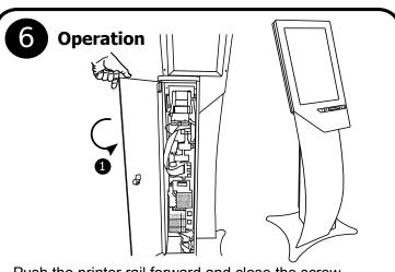
Push the printer rail forward and close the screw. Close the cover as shown in the picture (1) and lock the cover with Q-smart ticket machine key. Power On device.
