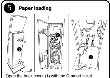
machine key. Unscrew the screw in section (2) and
