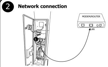
Connect the Ethernet output of the ticket machine to your modem, shown as (L) in the picture. You can find the IP address of the device on the screen when the application starting.
