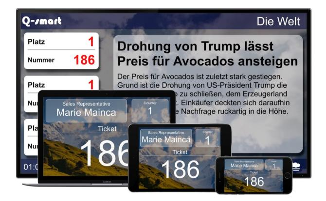
Cloud screens embedded in the queue management system can be used in the form of two different applications as the counter screen and main screen. Cloud screen is a Web-based application running on a built-in Web server.
